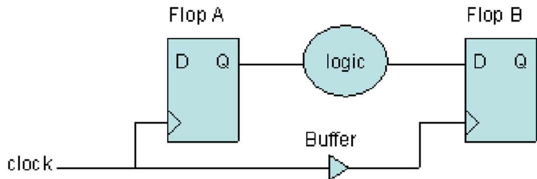
$$T_{launch} + T_{ck2q} + T_{dp} < T_{capture} + T_{cycle} - T_{setup}$$
